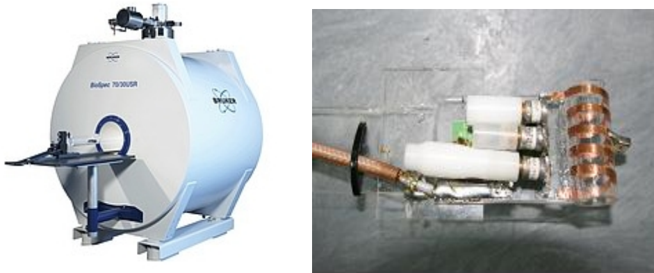
Fig. 2. Animal magnetic resonance imaging/spectroscopy (MRI/S) system at SBRI and a self-developed high-sensitivity radio-frequency (RF) coil for MRI/S systems.
